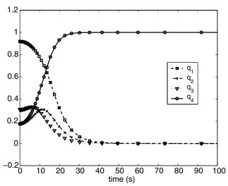
Fig. 8 Quaternions for the NPSAT1 stability problem; stars represents the discrete solution with 60 nodes and the solid lines are propagated trajectories.
